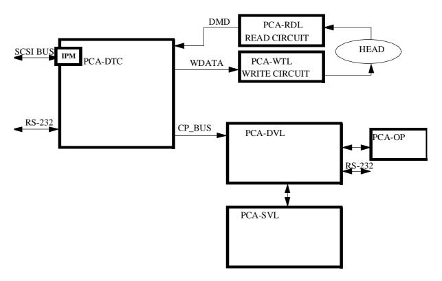
Figure 2-1. M2488 Block Diagram
